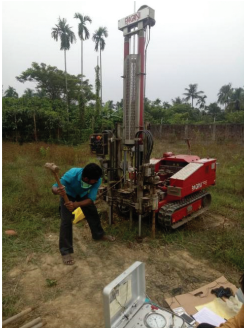
Figure 8. SDMT test in progress at the project site.
