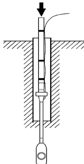
Figure 5.7. Torpedo assembly
