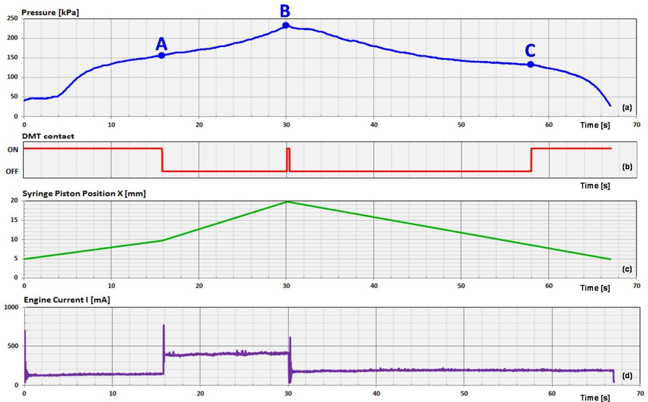
Figure 6.3. Example of data recorded in a full Medusa DMT test cycle adopting the standard DMT procedure: (a) pressure and A, B, C readings, (b) membrane contact status, (c) syringe piston position, (d) engine current. All data are plotted versus time, where  $t = 0$  corresponds to the instant when penetration stops and the test cycle begins.
