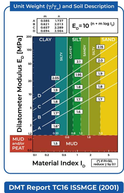
Figure 8.1. Summary of DMT data processing and interpretation formulae, adapted from ISSMGE TC16 Report (Marchetti et al. 2001). On the right: chart for estimating soil type and unit weight  $\gamma$  (normalized to unit weight of water  $\gamma_w$ ) from  $I_D$  and  $E_D$ , graphically modified version of the chart developed by Marchetti and Crapps (1981)
