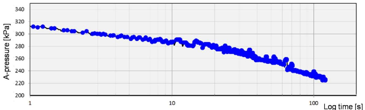
Figure 11.4. Detail of the A-pressure versus log time measurements during a short A-dissipation test prior to membrane expansion at the site of Cesano, Rome, Italy (same data as in Figure 11.3a, Marchetti et al. 2019)
