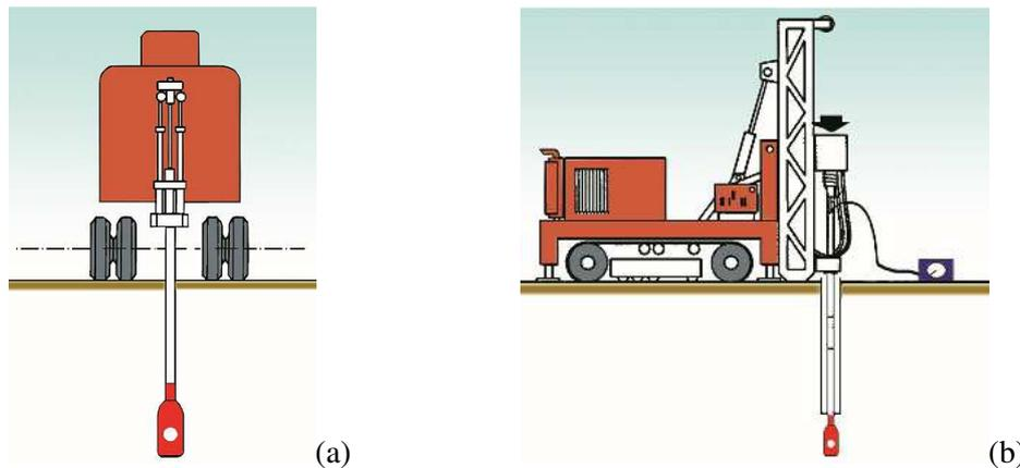
Figure 5.5. Thrust machines for advancing the Medusa DMT/SDMT: (a) truck penetrometer, (b) drill rig
