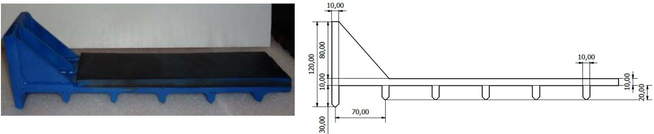
Figure 7.1. Example of shear beam for generating a shear wave
