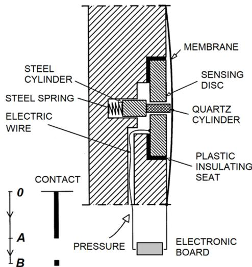
Figure 5.3. Detail of the operation mechanism of the dilatometer blade
