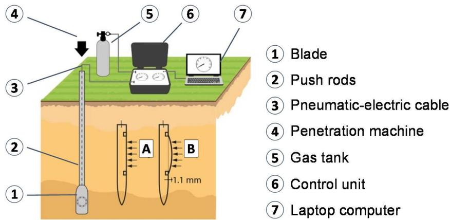
Figure 3.1. Main components of the traditional pneumatic DMT equipment and test layout
