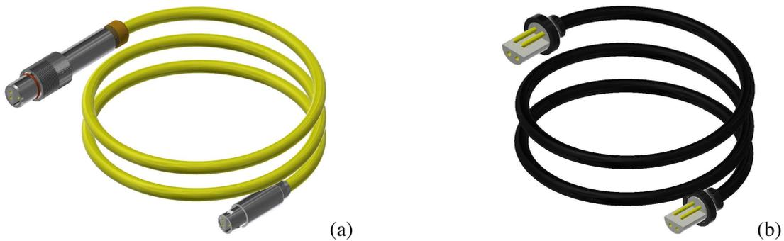
Figure 5.4. Electric cable: (a) cabled version, (b) cableless version
