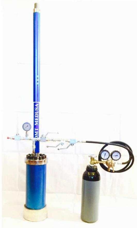
Figure 11.1. Calibration chamber used for preliminary tests on the Medusa DMT (Marchetti 2018)
