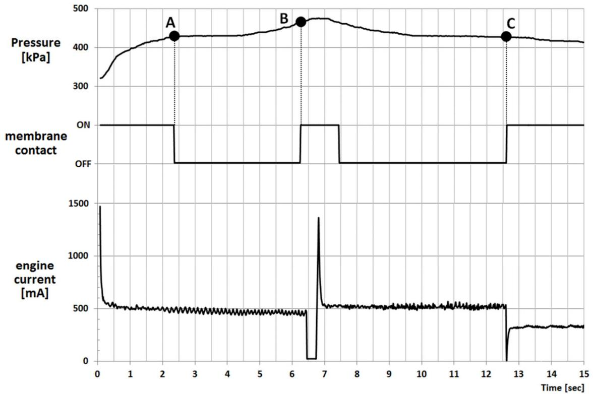
Figure 11.2. Diagram of pressure, membrane contact status and engine current versus time in a full DMT cycle using the Medusa DMT in the calibration chamber pressurized at about 450 kPa (Marchetti 2018)
