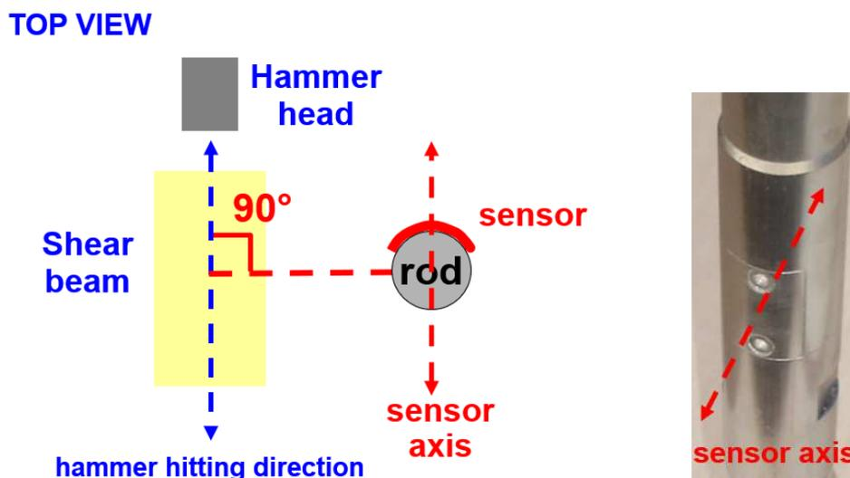
Figure 7.2. Correct orientation of shear beam and sensor axis
