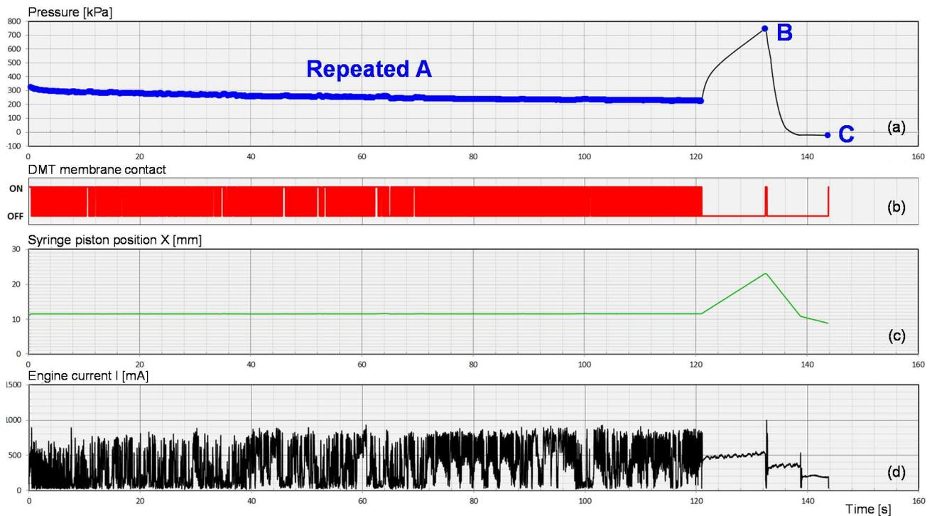
Figure 11.3. Results of a short A-dissipation test prior to membrane expansion obtained by Medusa DMT at the site of Cesano, Rome, Italy (Marchetti et al. 2019): (a) pressure and A, B, C readings, (b) membrane contact status, (c) syringe piston position, and (d) engine current. All data are plotted versus time ( $t = 0$  when penetration stops and the test cycle begins).
