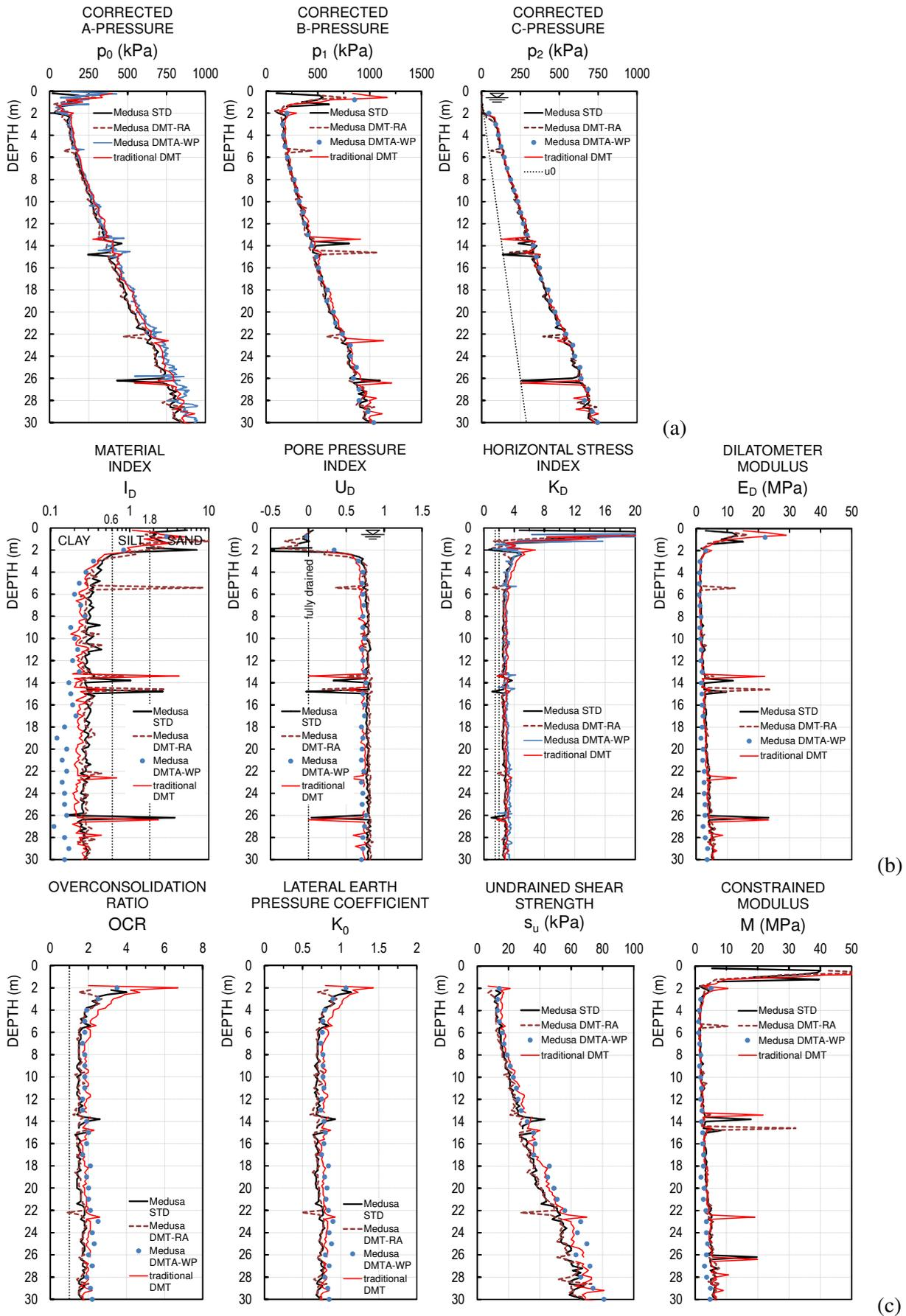
Figure 12.1. Comparison of results obtained by Medusa DMT using different test procedures and by traditional DMT at the research test site of Fucino – Telespazio (September 2020)
