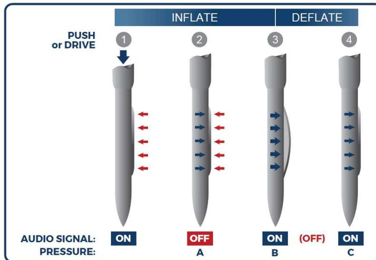
Figure 6.2. Sequence of the standard DMT procedure
