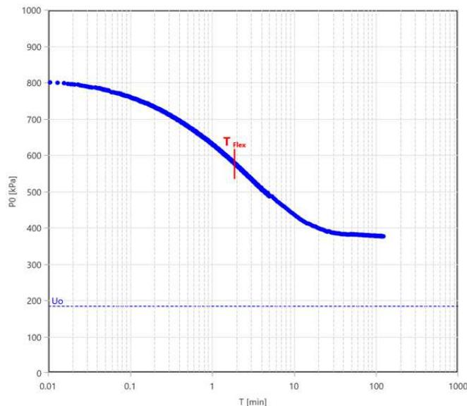
Figure 6.5. Sample dissipation curve obtained with the Medusa DMT (ELI ALPS – Szeged, Hungary, November 2020)
