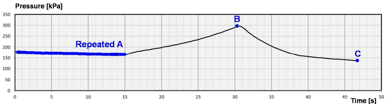
Figure 6.4. Full test cycle obtained by DMT Repeated *A*-readings procedure (DMT-RA) at the research test site of Fucino – Telespazio (September 2020), sounding Medusa 2, depth 8.0 m
