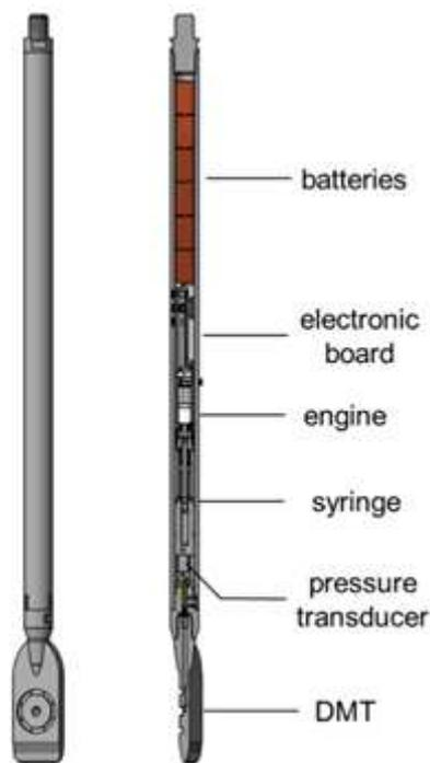
Figure 5.1. Main components of the Medusa dilatometer
