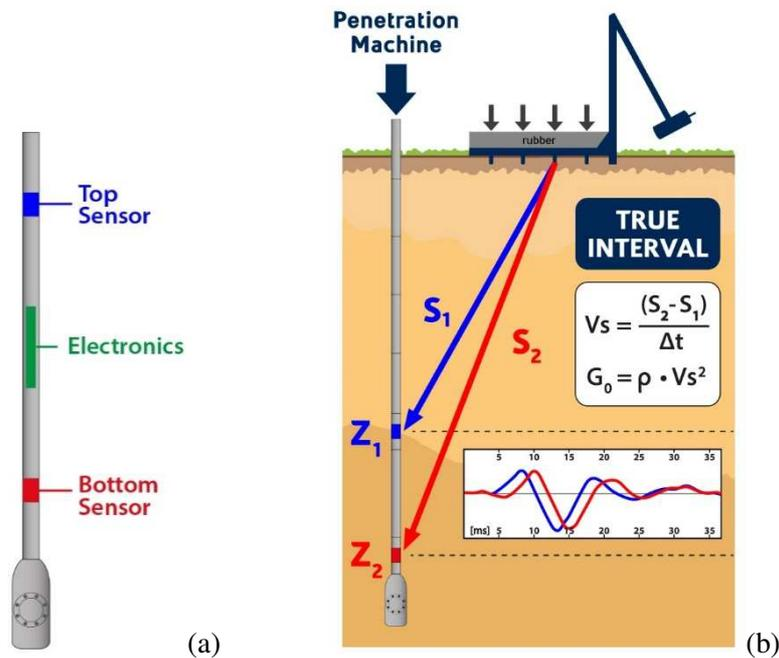
Figure 3.2. Seismic dilatometer equipment (a) and test layout (b)
