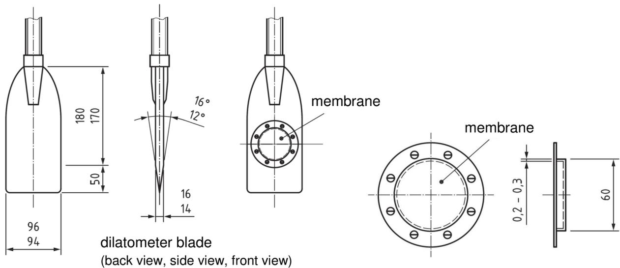
Figure 5.2. Dimensions of the dilatometer blade and membrane (ISO 22476-11:2017(E))
